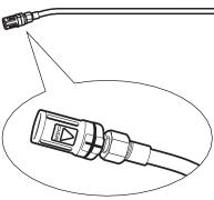
**Step 1** To apply detergents the triple jet nozzle must be set to the "CHEM" position.
